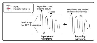
Use the [Input Level Button] to adjust the volume so that the [PEAK Indicator] does not light up even when the loudest sound is produced by the target. Doing this prevents clipping during the loudest parts of a song or during instrumental passages played fortissimo.
